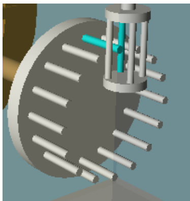
Figure 4: The cyan pegs on the crown and pinion are a visual aid to see that the pinion rotates four times for every single time the crown rotates.
