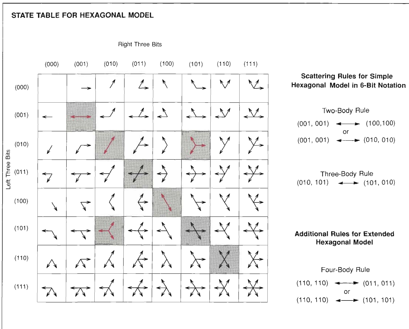
Fig. 5. All possible states of the hexagonal lattice gas are shown in the state table. Each state can be expressed in 6-bit notation (a combination of 3 right bits and 3 left bits). For example, the empty state is written (000,000)
