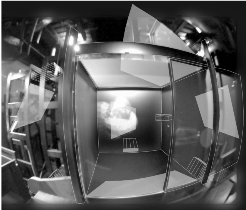
Fig. 1. A fisheye view of the ALICE VR theater, highlighting five of the six mirrors and projectors. The view is from near the sixth projector, which aims at the sliding door (halfway open in this photograph).
