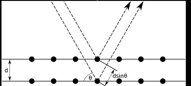
The extra distance traveled by the bottom wave has to be an integer multiple of the wavelength,  $\lambda$ .
